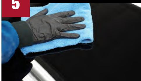
Wipe clean with **Ultra Microfiber Towel** and visually inspect to ensure defect has been removed and polished to a gloss.
