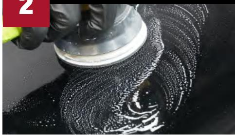
Further refine sand-scratches with 3000-grit foam pad and water on a 3" DA sander.
