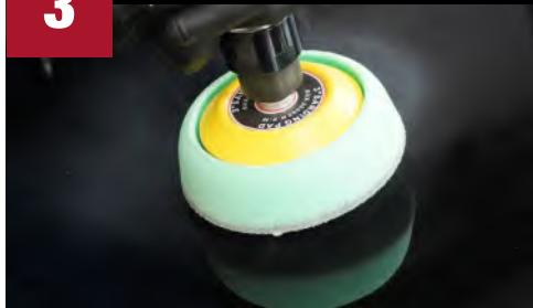
Compound the area using **Performance Cutting Compound** on a **3" Green Foam Pad**.
