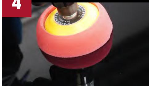
Polish the area using **Performance Finishing Polish** on a **3" Red Foam Finishing Pad**.
