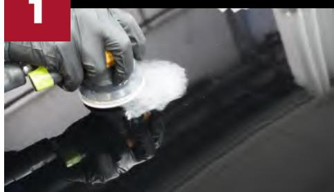
Remove paint defects using 1500-2000 grit sandpaper on a 3" DA sander.
